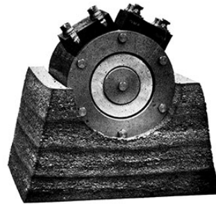
Fig. 1. The Magnetophone supported on its cushion of sponge rubber.
