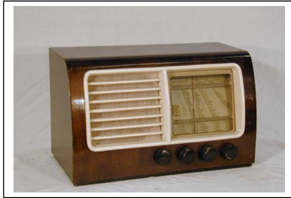
Bang & Olufsen (B&O) MINI 43 (1943) Valvole: UCH4- UCH4- UBL1- (foto dal Danish Museum of Electricity ( www.elmus.dk ))
